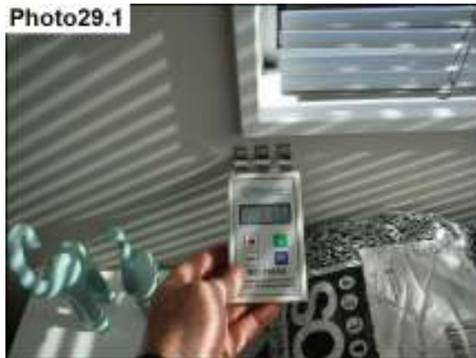
Moisture reading in bedroom 2. 11.6%
